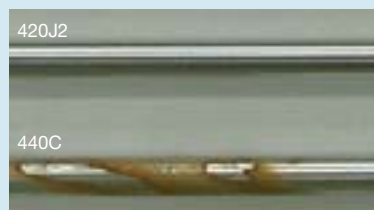
Immersion test in 5% saline solution for 24 hours
